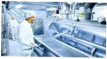
The state-of-the-art, semi-automated blending line can be used flexibly for order sizes from 500 lbs. to over 22,000 lbs. It features high blending precision of up to 1:100,000, fast setup times and flexible filling into small or large containers. Photo courtesy of SternMaid.
